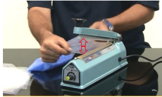
Step 4. Place Bag in between the silicone and seal bar then press down
