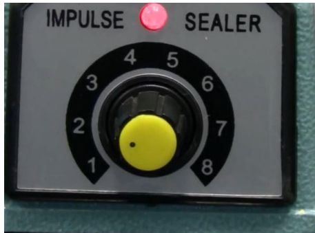
Step 5. Make sure that the Red light indicator turns on when pressed down then turns off which means that the seal is done
